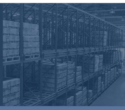
Racking system is a special system for shuttle which is based on the structure of Drive-in racking. It is suitable for storing goods of large quantity by small varieties, such as food, fruits, chemicals, tobacco industry. It is also the best choice for cold operation storage.
